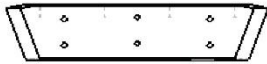
H11 | SOLIVE DE TOIT - W4L14438 (1) | 1 po x 3 3/8 po x 15 15/16 po (24 x 86 x 404)
