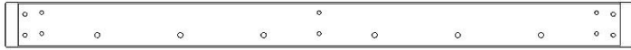
H02 | SOLIVE DE TOIT - W4L14430 (1) | 1 po x 3 3/8 po x 46 3/4 po (24 x 86 x 1 188)
