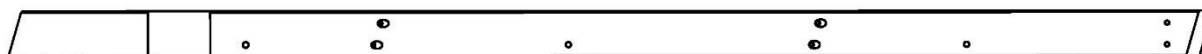
H09 | SOLIVE DE TOIT - W4L16214 (2) | 1 po x 3 3/8 po x 88 1/8 po (24 x 86 x 2 240)
