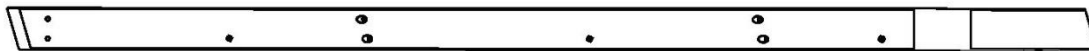
H01 SOLIVE DE TOIT - W4L16213 (1) 1 po x 3 3/8 po x 88 3/16 po (24 x 86 x 2 240)
